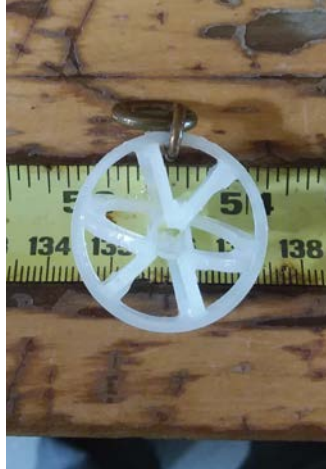
Figure 3. Image of a BioRing used to simulate catch in the scale survey dredge. Each BioRing either had a weight in the center of the ring or weight attached to the outside of the ring, as shown in this picture.
