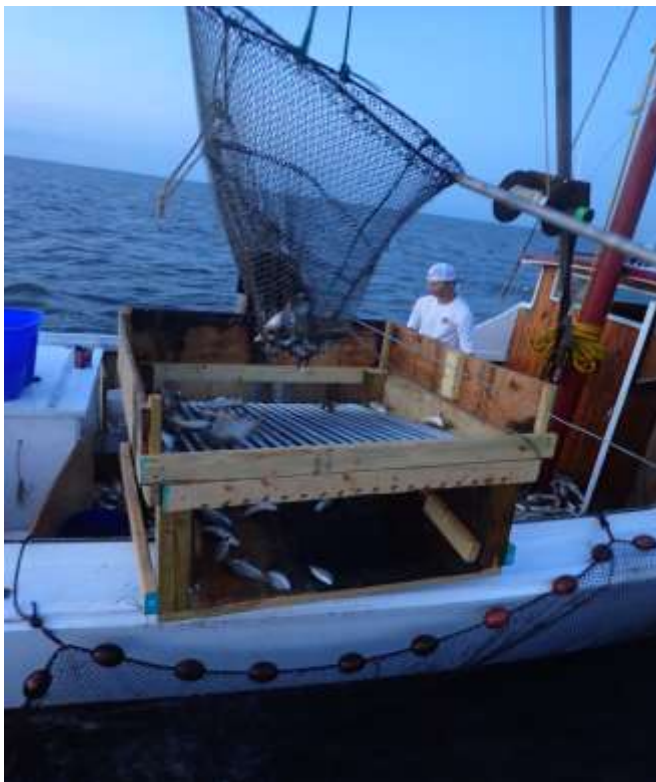
Figure 3. Fish culling table actively separating fish by size. The spacing and slope of pipes were adjusted to improve culling.
