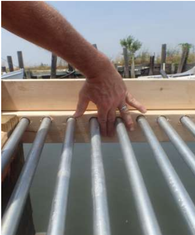
Figure 1. Cull table used showing initial spacing of metal pipes (grating) designed to allow small fish to pass through.
