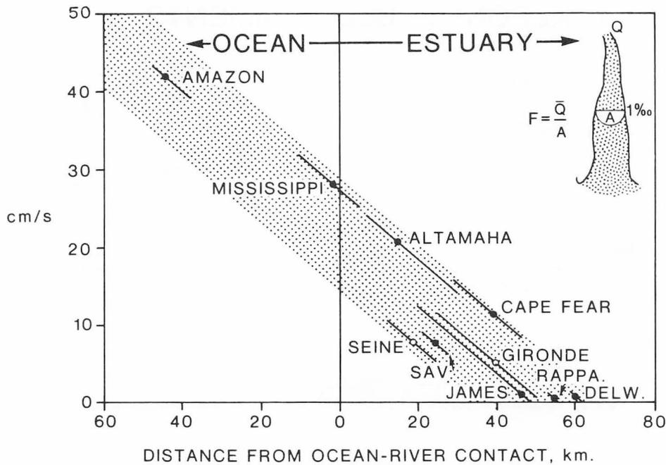
Figure 5. Position of the inner limit of salty water at 1 ppt salinity in relation to flushing velocity for various river estuaries. Length of line represents seasonal range in position; dots and circles indicate position at average river inflow. Sav. is Savannah; Rappa. is Rappahannock estuary; Delw. is Delaware estuary. Inset:  $F$  is flushing velocity;  $\bar{Q}$  is average river discharge; and  $A$  is cross-sectional area at landward limit of salty water. Adapted from Gibbs (1977).
