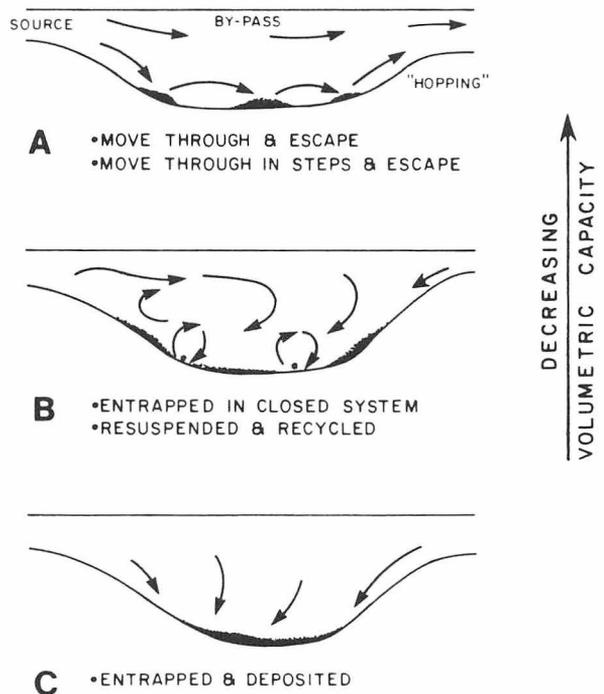
Figure 2. Cycling modes and fate of suspended sediment in an estuary. Arrows represent pathways of sediment dispersal; schematic.
