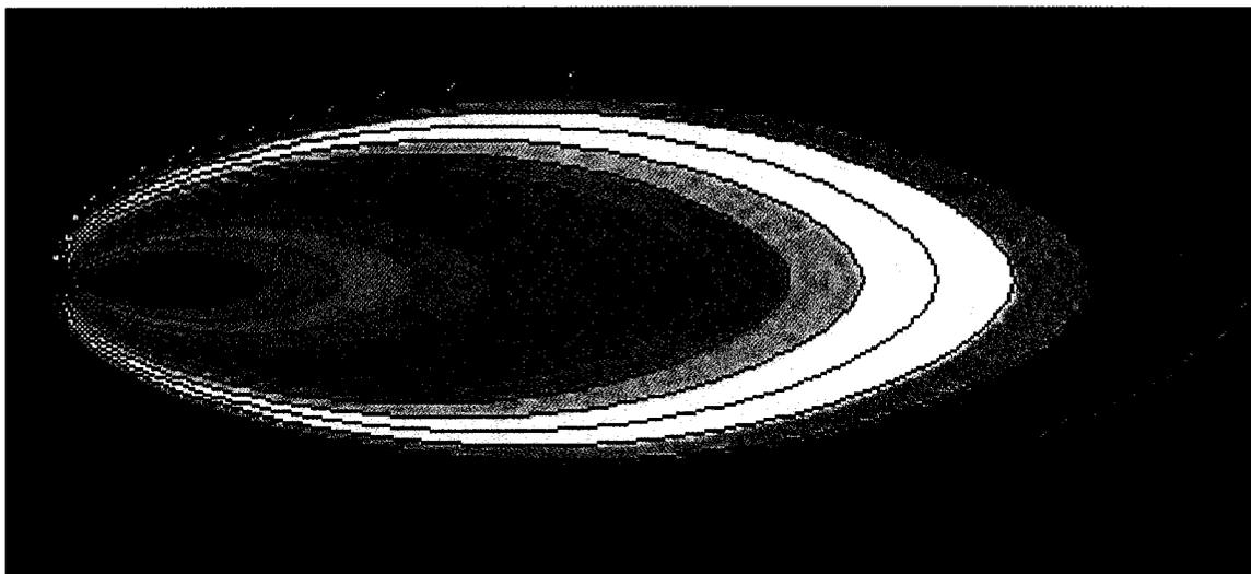
Figure 3-23. Cellular automata fire spread contours depicting fire boundary locations. The simulation used a wind angle of 90 degrees and a length-to-breadth ratio of 2.0, for 500 iterations. Unequal weighting factors create an elliptical fire spread shape typical of an actual fire in wind driven conditions.
