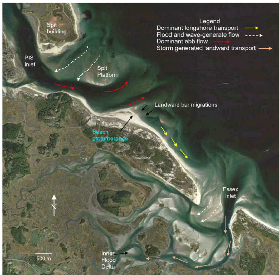
Figure 15. Conceptual model of sand transport pathways at the study area. This conceptual diagram traces the pathway of sand transport from southern Plum Island to Essex Bay. A description of the mechanism and sand reservoirs is described in the paper.
