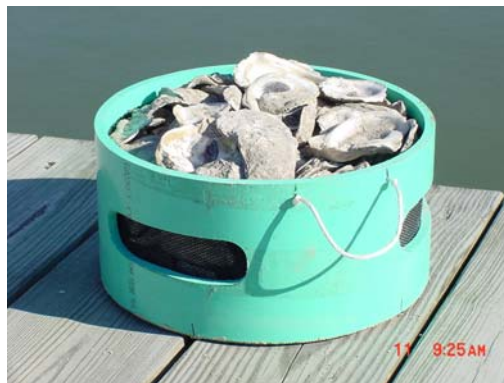
Figure 9. Substrate basket used for sampling reef resident fish and decapods.
