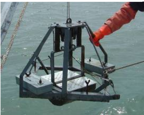
Figure 2. Smith-McIntyre grab sampler.
