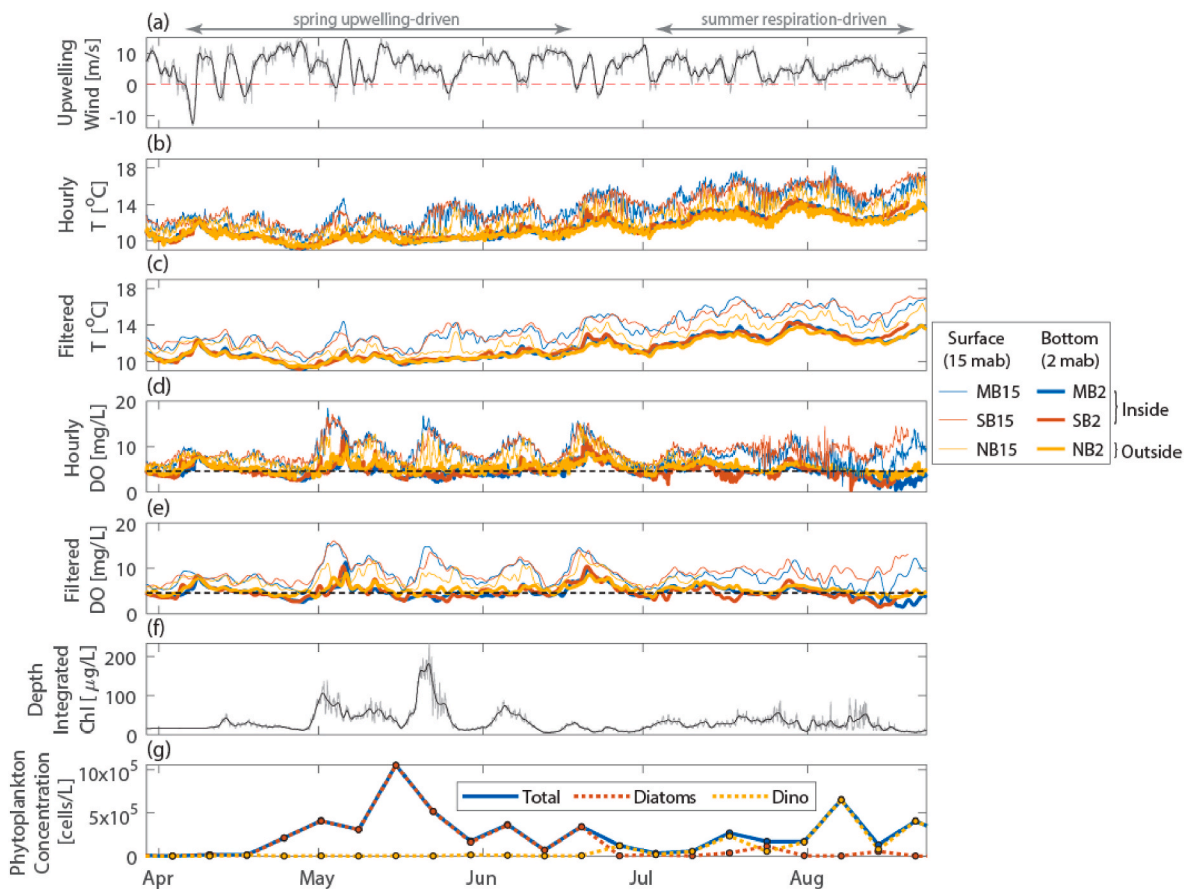
Fig. 2. Time series from late March to late August. (a) Upwelling favorable winds, with the hourly (gray) and low-pass filtered (black) data. (b) Hourly temperature, (c) low-pass filtered temperature, (d) hourly dissolved oxygen, and (e) low-pass filtered dissolved oxygen at each mooring (Outside Bay: NB – orange; Inside Bay: MB – blue and SB – red). The thick lines in the panels b–e correspond to the near-bottom (2 mab) measurements, while the thin lines denote the near-surface (15 mab). The dashed line in panels (d) and (e) represents the hypoxic threshold of 4.6 mg/L. (f) Depth-integrated chlorophyll measured from the Cal Poly Pier profiler and the low-pass filtered quantity (black). (g) Surface phytoplankton concentration and community composition from inside the bay at the Cal Poly Pier. Nearshore sites MB and SB are inside the bay and NB is outside the bay (Fig. 1). The light gray arrows at the top denote the approximate timing of the two hypoxic regimes identified (Section 4.1). (For interpretation of the references to color in this figure legend, the reader is referred to the Web version of this article.)
