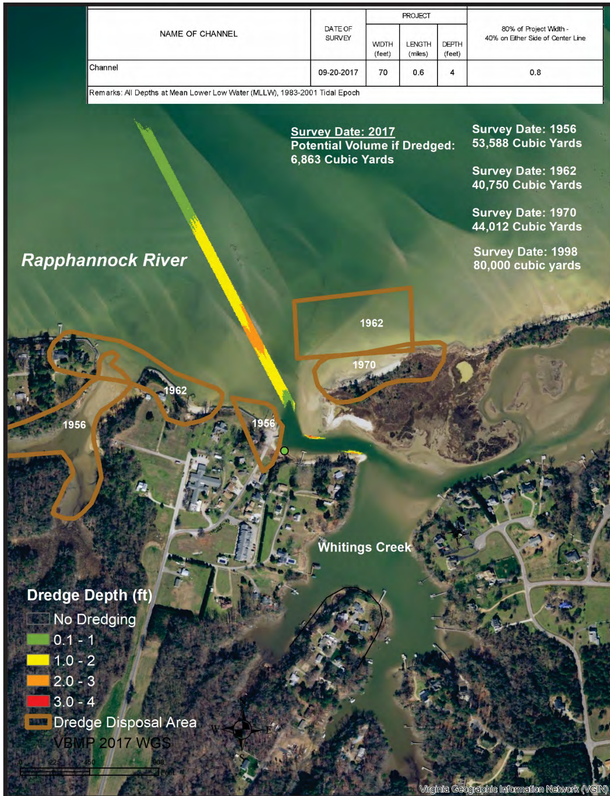
Figure 11. Whiting Creek federal channel in Middlesex County showing the amount of material that needs to be dredged from the channel as well as precious dredge cycles and disposal areas. From Hardaway et al. (2019).
