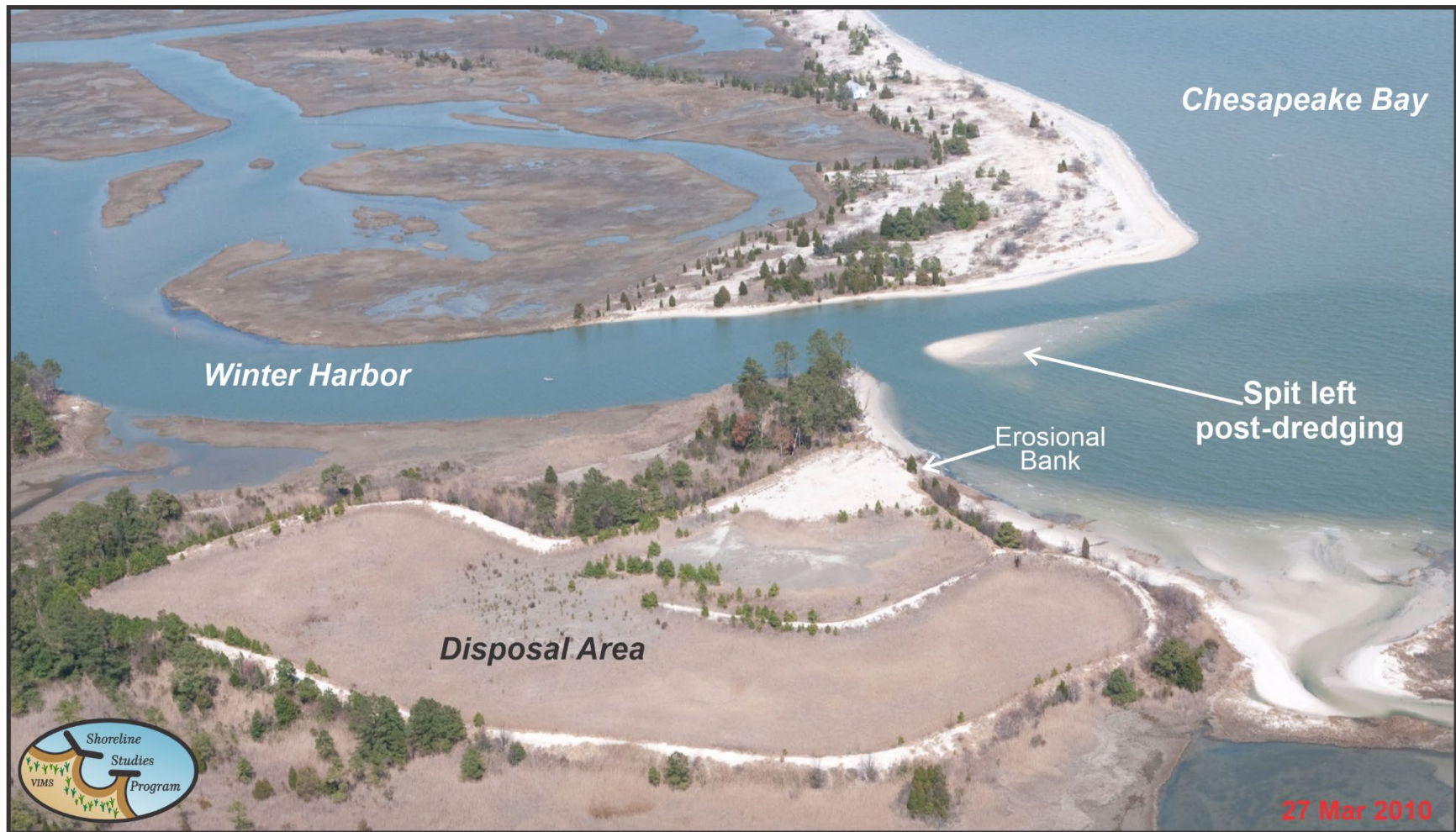
Figure 7. Aerial photo of Winter Harbor Inlet, post dredging in 2010. The material was placed to the north. Only the Federal channel was dredged; the sandy spit south of the channel was left in place.
