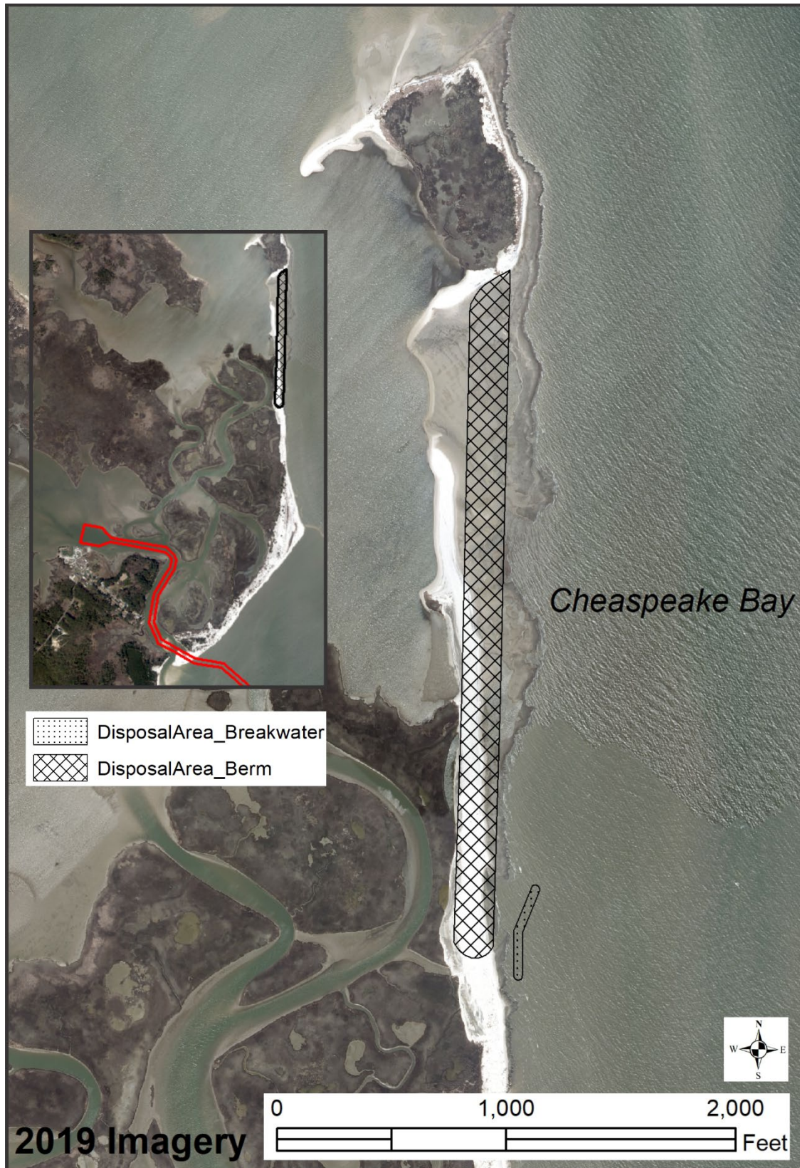
Figure 22. Proposed placement for sandy material beneficial use and proposed nearshore breakwater. The inset shows location relative to the channel. Pumping distance is about 1.5 miles.
