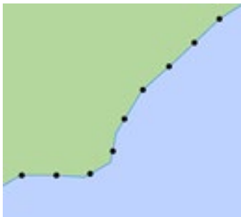
Figure 4. The black dots represent the midpoints of 10m segments along the shoreline. Initial step in building Thiessen polygons to model wetlands migration.
