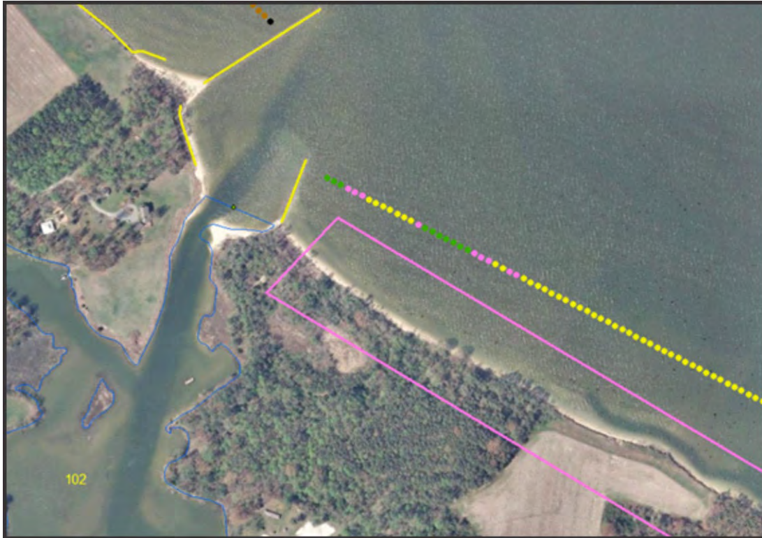
Figure 3-5. Structures mapped at Bonum Creek, and shoreline change rates downdrift of the creek identifying potential dredge material placement areas.
