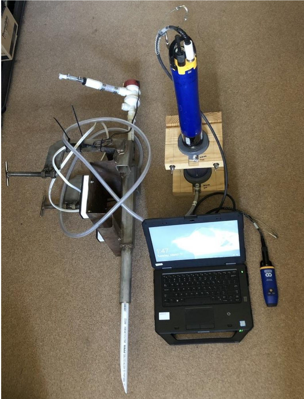
Figure 4-1 Data flow setup. Transom mount hydraulic ram and bilge pump (left) to send water to a YSI EXO2 Sonde with a flow cell held in a wooden bracket (upper right), cabled to an EXOGo GPS antenna and data integrator (lower right) to send georeferenced sonde data to a laptop by bluetooth.
