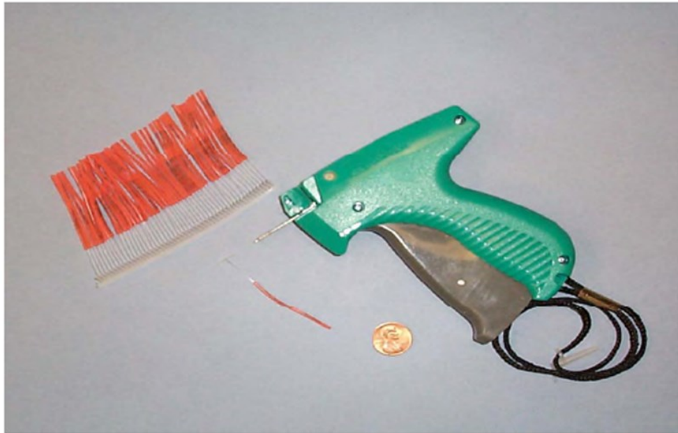
Tagging Gun and T-Bar Tags (top photo); Stainless Steel Dart Tag and Applicator (bottom photo) (Note: coin for scale – 0.75 inches diameter)
