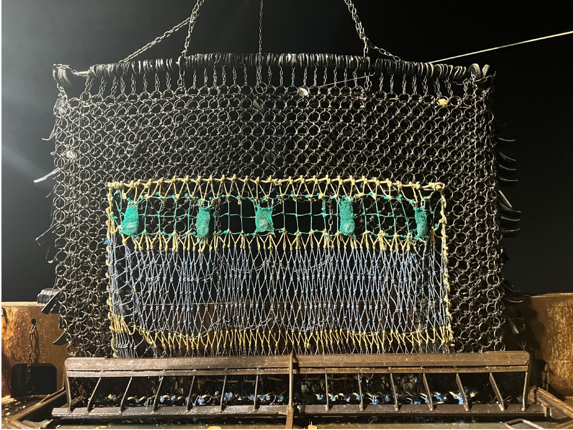
Figure 4. Image of the Pisces light attached to the experimental twine top square mesh escape panel located at the bottom of the twine top referred to as SMVP2 in the attraction configuration.
