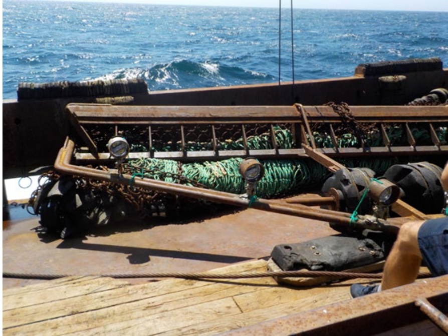
Figure 2. Image of the Pisces light attached to the balebar of a dredge in the deterrent configuration.
