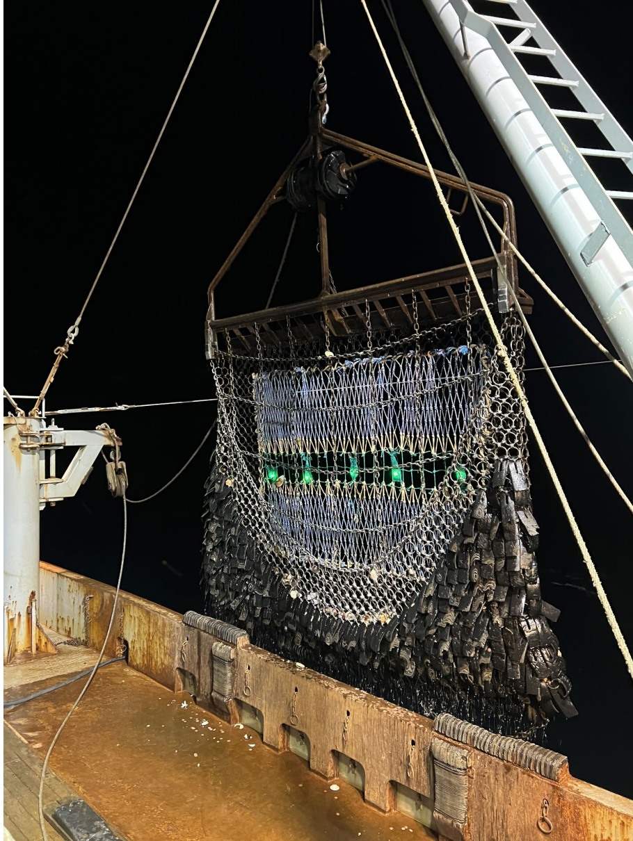
Figure 3. Image of the Pisces light attached to the experimental twine top square mesh escape panel located in the middle of the twine top referred to as SMPV1 in the attraction configuration.
