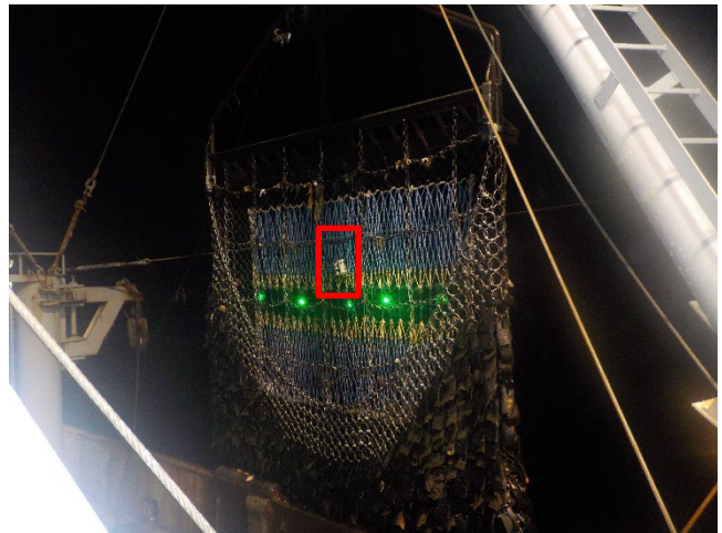
Figure 5. Images of the Pisces CatchCam system. The entire system is in the top left. The system attached to the dredge frame looking out from the dredge is in the top right. Examples of how the system was attached to the experimental twine top are shown in the bottom two photos (outlined in red).
