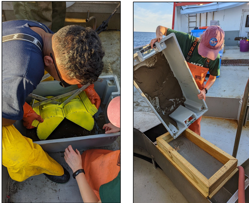
Figure 13. (Left) Petersen grab sample collection. (Right) Benthic sediment sample is collected and placed into a bin. Sample is then sieved through mesh and retained for lab processing.
