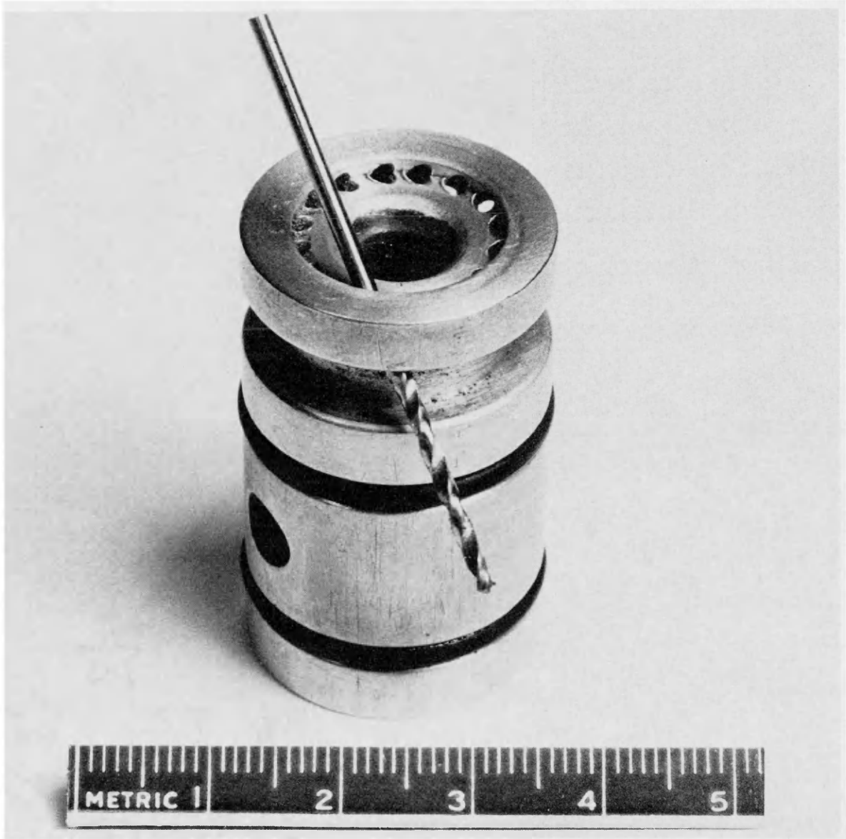
Figure 10.- Spiral water flow assembly used to water cool and hold silicon disc into sample probe.
