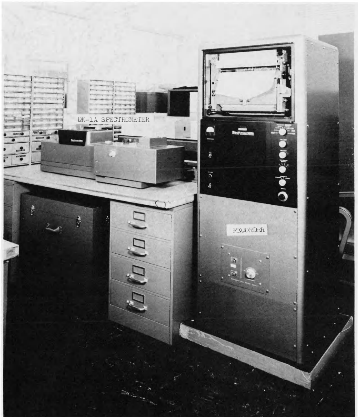
Figure 6.- DK-1A spectrometer used for making transmission spectra from 0.75 - 2.5 microns.
