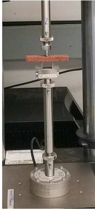
Figure 14. Flexural test setup on the Instron 5848 Micro Tester.
