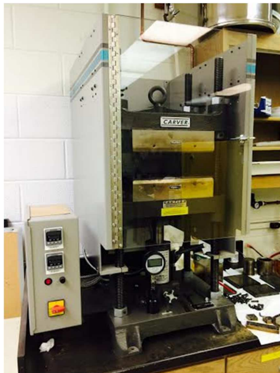
Figure 11. Heated hydraulic press experimental setup.
