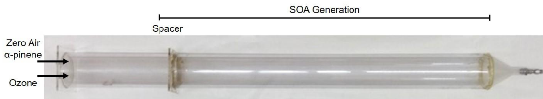
Figure 5 Polycarbonate flow tube for IRMPD SOA generation.
