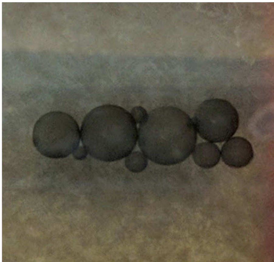
Figure 1.10: Optical image of graphene coated bubbles of water in heptane. Since the heptane and water are immiscible liquids, they remain separated when combined in a single vessel. The interface between the two liquids is the most energetically favorable location for the graphene sheets, which do not readily suspend in either solvent. When graphite is combined with heptane and water in a sealed vial and the vial is shaken, the graphite exfoliates to better cover the interface and graphene coated bubbles result. Bubbles are visible to the eye and are in the millimeter range.
