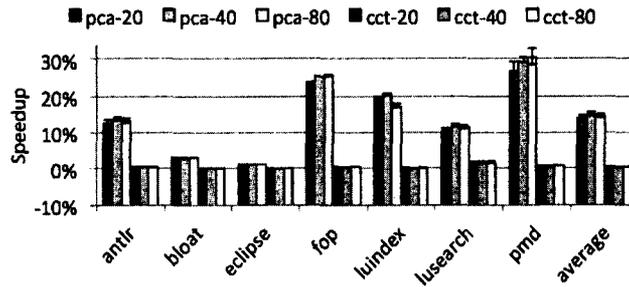
Figure 5.11: Speedup when call sequence prediction is used for parallel JIT compilation (Two compilation threads are used).
