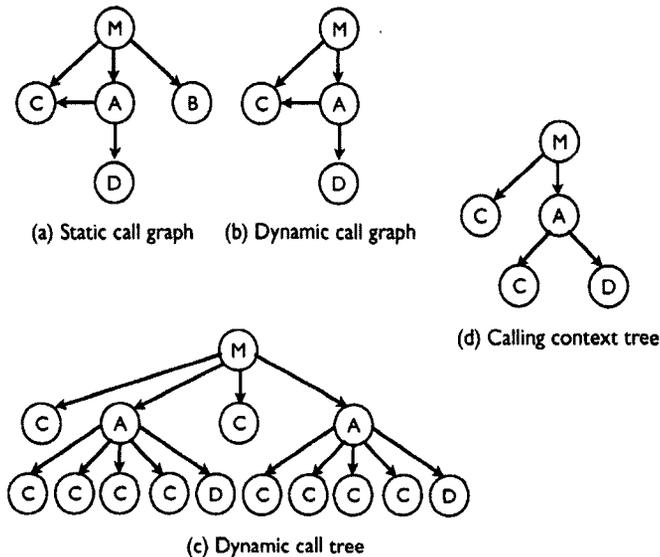
Figure 5.7: Four other representations of function calls in executions of “PCAExample” in Figure 5.1 (a). In the program, no functions except “M” and “A” contain function calls. In the considered execution, the “if” branch is taken.
