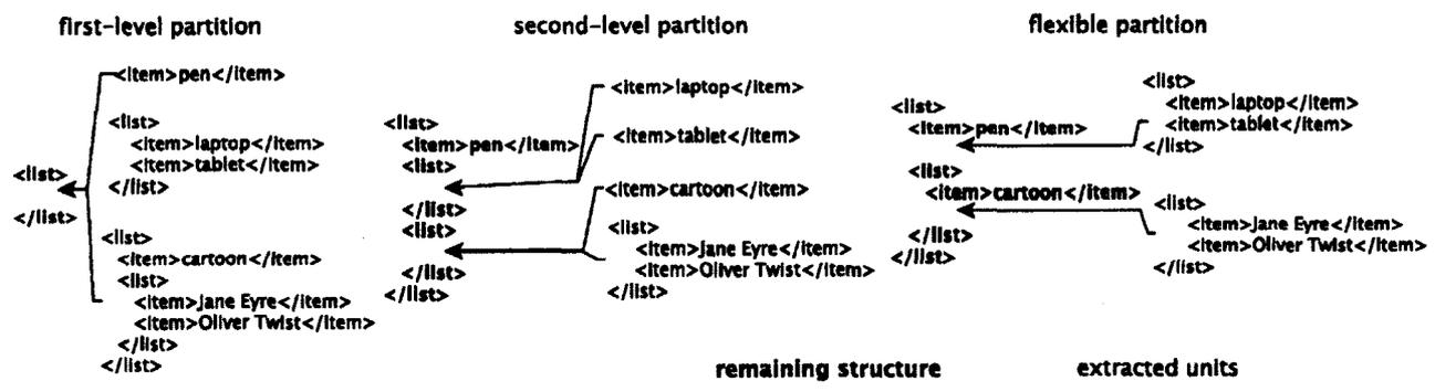
Figure 4.7: Partitioning strategies in the partitioning-oriented scheme. Partitioning results of the input in Figure 4.6 through three different partitioning strategies in the partitioning-oriented scheme (bold font for remaining structures and normal font for extracted units).
