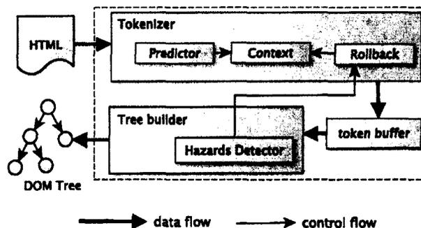
Figure 4.4: The speculative pipelining framework for HTML5 parsing.
