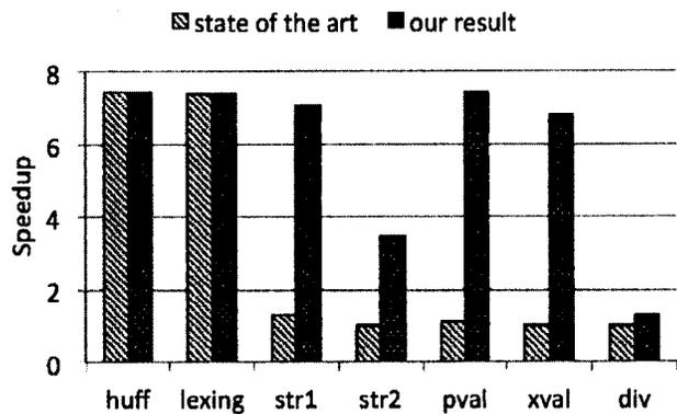
Figure 2.2: Speedups Comparison between the state-of-the-art and ours. The speedups brought by the state-of-the-art speculation scheme [90] are limited on some complex FSM applications. The results are for 8 threads running on an 8-core machine. Details are shown in Section 2.6.
