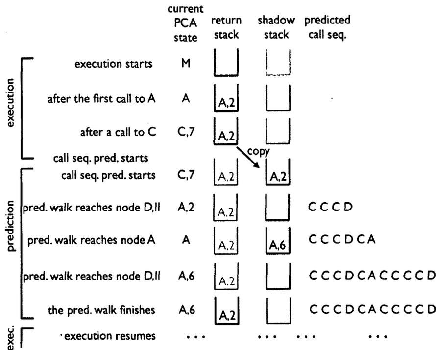
Figure 5.3: Illustration of how the PCA in Figure 5.1 (b) supports call sequence prediction. It assumes that the prediction starts after execution sees the call sequence “M C A C” and the goal is to predict all remaining function calls.
