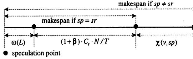
Figure 2.4: The make-span of a thread.
