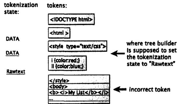
Figure 4.3: A failure of naive pipelined HTML parser. An example showing that the naive pipelined HTML5 parser emits incorrect tokens, marked with underlines.
