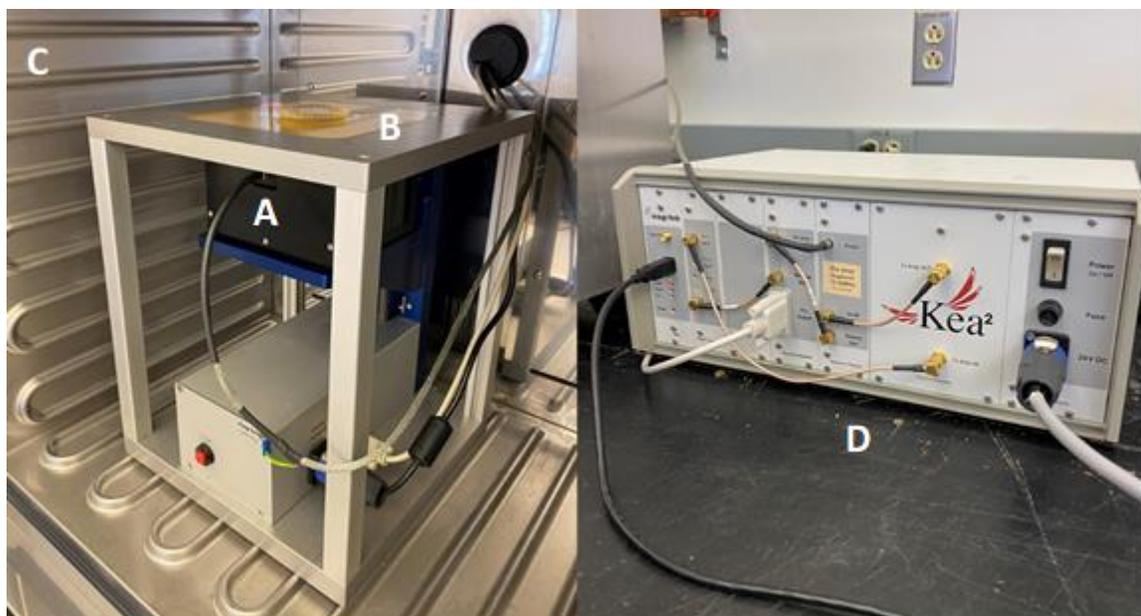
**Figure 11:** The PM5 NMR-MOUSE apparatus used in our lab. (A) The PM5 magnet (black) mounted onto the mechanical lift (blue) with aluminum housing and frame. (B) The sampling area for the magnet with a cured bulk epoxy sample sitting on top of the sensitive region. (C) The climate chamber that housed the PM5 NMR-MOUSE for temperature controlled real-time epoxy cure kinetic experiments (see Chapter 6). (D) The Kea2 spectrometer.
