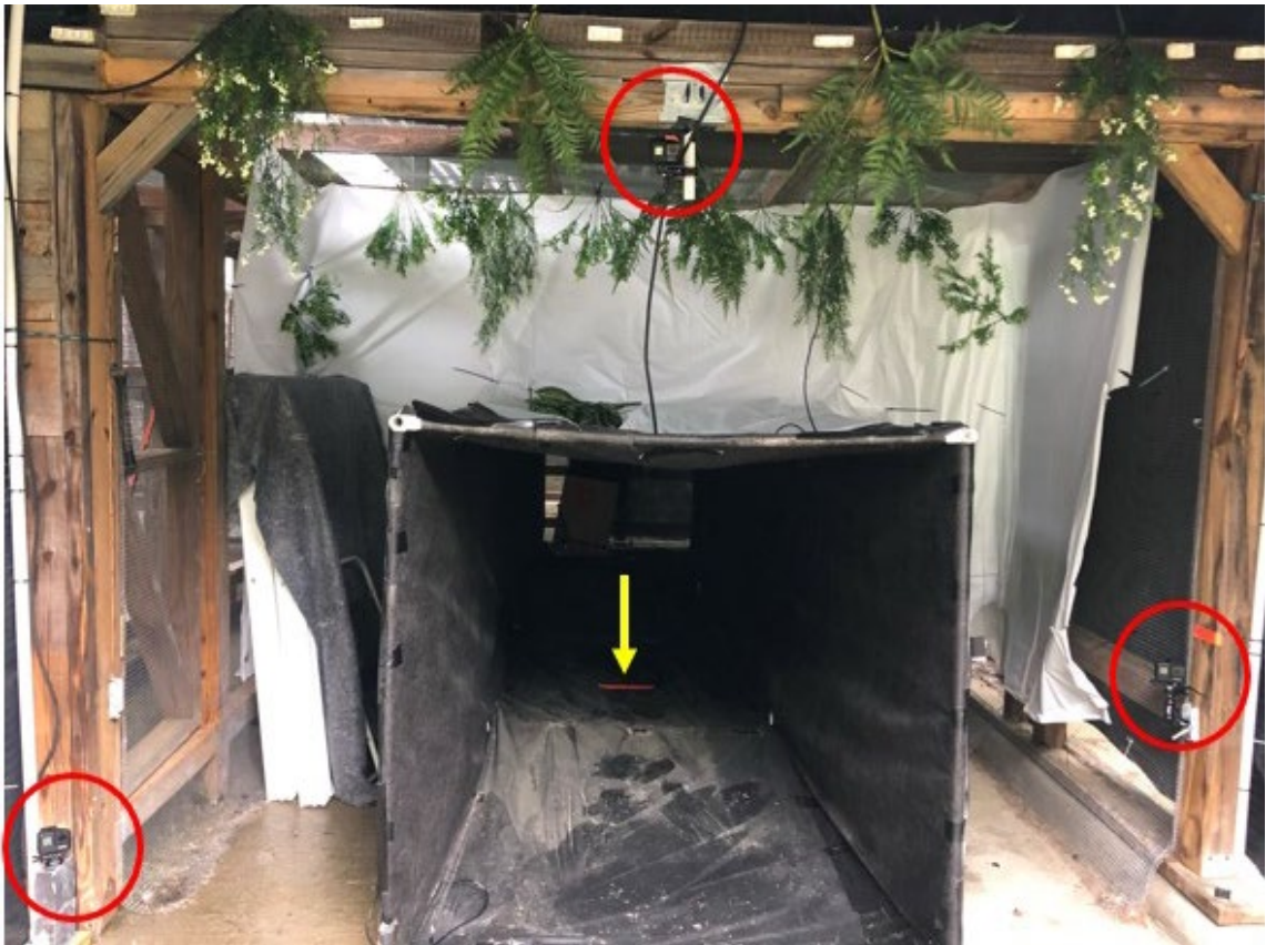
Figure 4. Camera set-up. Three GoPro HERO7 Black cameras captured flight behavior in the 4 m active section of the flight tunnel. Cameras were situated in a triangular formation, with the two lower cameras being slightly offset in order to capture the most comprehensive view of each flight. The starting point of each flight is indicated on the image with a yellow arrow.
