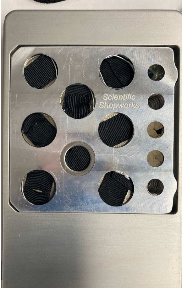
Figure 7: Customized tray for LA-ICP-MS analysis allowing for multiple samples to be scanned during each run.
