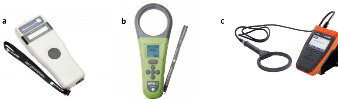
Figure 6: (a) GPR Plus Handheld PIT Tag Reader. Records time, date, tag number. Not waterproof. Unit cost $650 (Biomark). (b) HPR Lite Handheld PIT Tag Reader. Records time, date, tag number. Waterproof and shock resistant. Unit cost $950 (Biomark). (c) HPR Plus Handheld PIT Tag Reader. Records time, date, tag number, geographic position. Unit cost $3,670 (Biomark).
