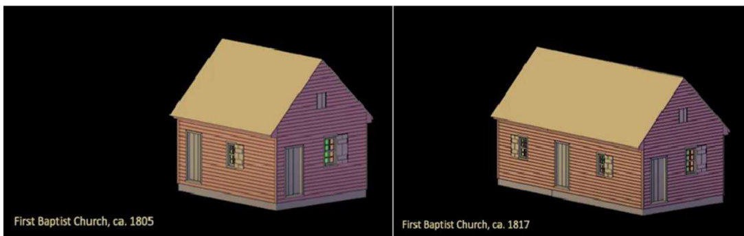
Figure 1: Architectural renderings showing the two-stage construction of the original Nassau Street church. Image from Colonial Williamsburg (2022).
