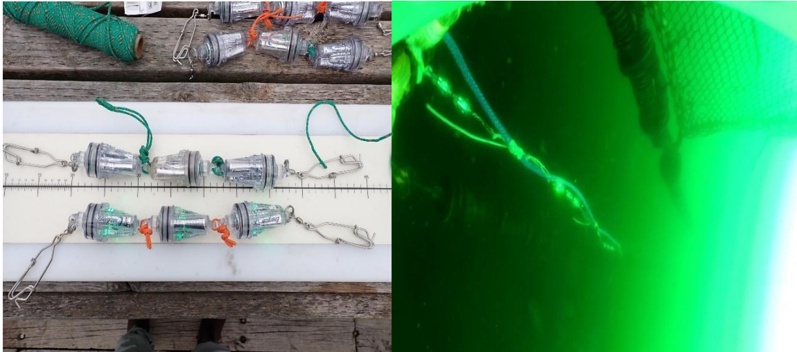
Fig. 2. (Left Photo) Electrolume LEDs tied together in groups of three with snaps attached to either end for easy attachment and removal between tows. (Right photo) Five LED clusters were attached to either side of the trawl along a 2.4-meter-long spectra rope that ran from the breastline to a hammerlock that connected the footrope extension to the beginning of the lower bridle. The photo was taken as the gear was being deployed.
