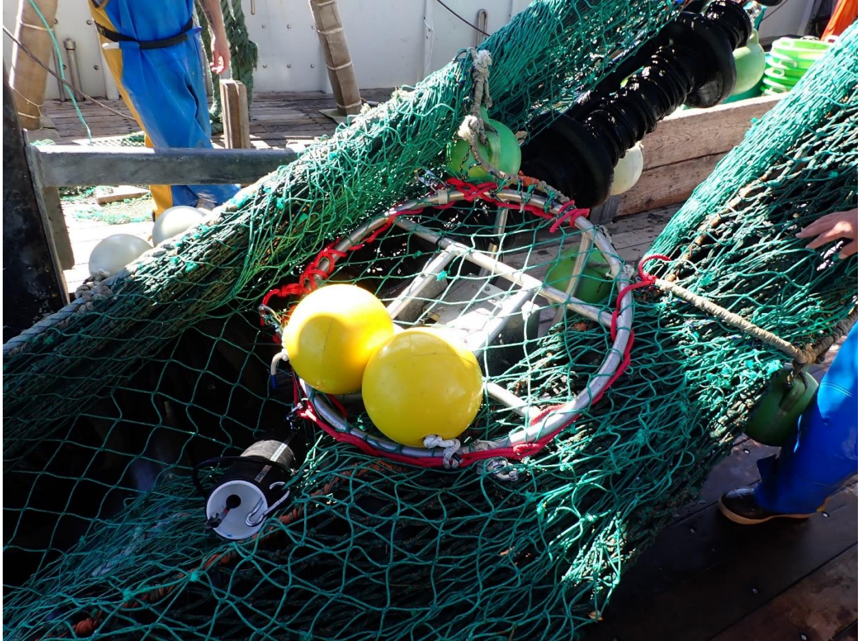
Fig. 2. DIDSON (Dual-frequency IDentification SONar) imaging device and apparatus centered on the top panel and focused on the port wing.
