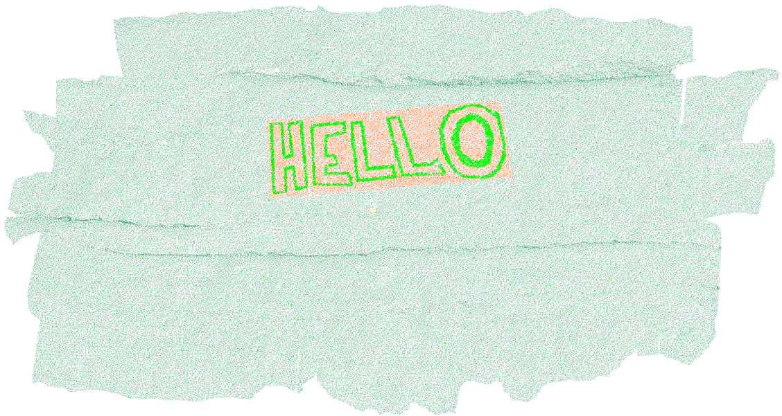
Figure 36: Sample E analysis. The sampled points [neon green] inside the inner rectangle [orange; 15,826 points] comprise 22.25% of the Master Cloud, whereas outside of this area [teal; 205,913 points] the remaining sampled points [215] amount to only 0.10% of the Master Cloud.
