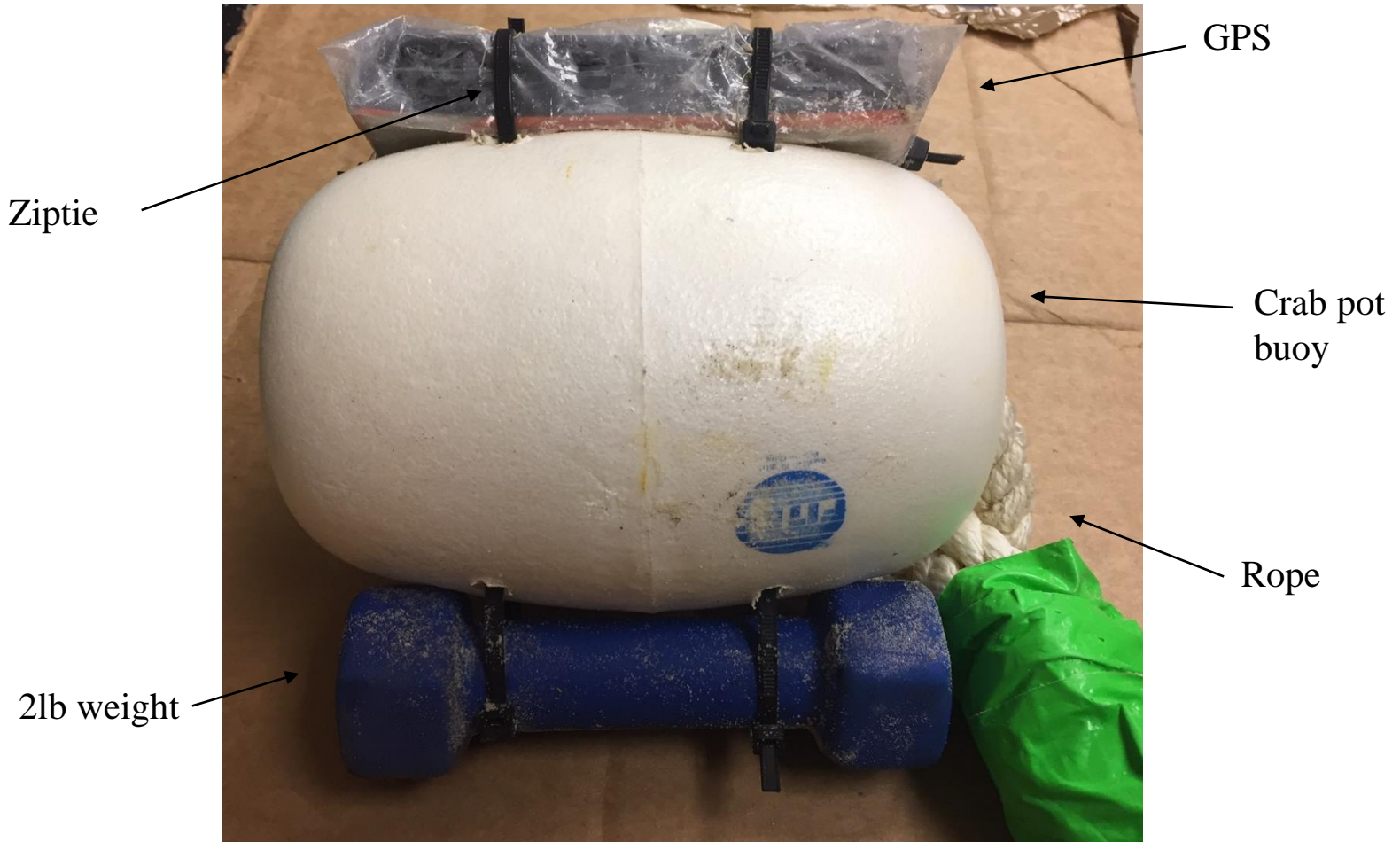
Figure A3. Self-righting buoy attachment with GPS for wood-foam and turtle carcass drifters.
