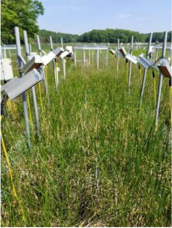
Fig. S1. SMARTX transect showing aboveground infrared heaters (foreground) and open-top elevated CO 2 (eCO 2 ) chamber (background). Heating cables extend 1.5 m into the soil and are located every 50 cm.
