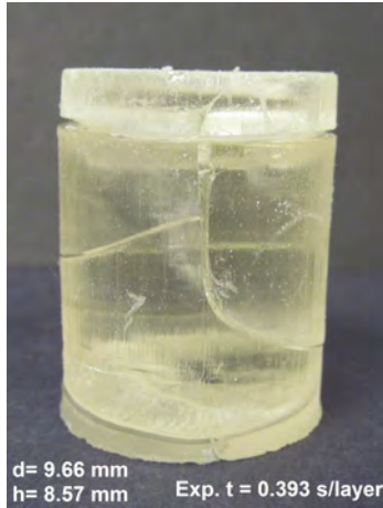
Figure 8: Large internal cracks evident on a print with PMT-compatible dimensions. These cracks developed days after the print was printed and cured for 20 minutes with an ultraviolet lamp. Repeated prints cured for only 5 minutes also developed internal cracks similar to these.
