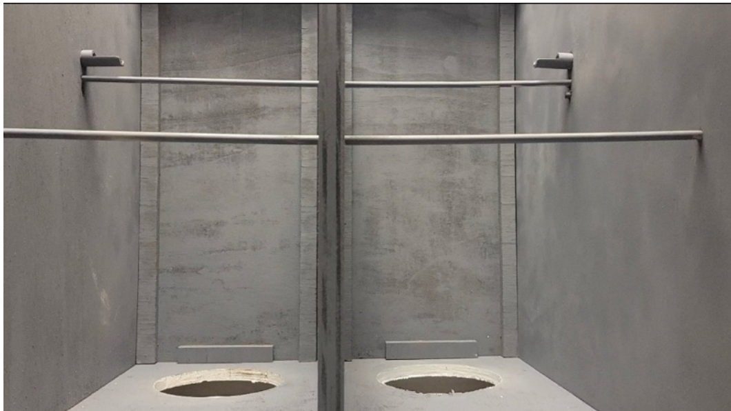
Figure 2. A schematic (a) of the testing area and a front interior view (b) of the area as photographed from the perspective of the release box. The middle line represents a separation between the left and right chambers. The circular openings were used to present the polarization cues, which were recessed under
