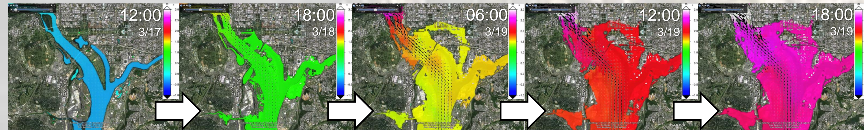
Figure 4. Great Flood of 1936 inundation displayed in Google Earth with depth-averaged velocities at 5 different times leading up to the peak of maximum inundation (12:00 on 3/17, 18:00 on 3/18, 06:00 on 3/19, 12:00 on 3/19, and 18:00 on 3/19)
