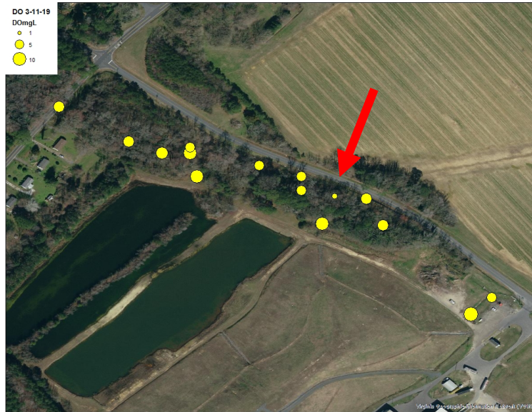
Figure 1. Identification of a groundwater discharge area by low dissolved oxygen recording in 2019 (red arrow).
