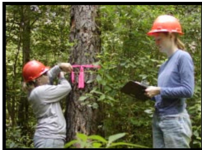
Field technicians Danni Larson and Sandra Smith measuring the DBH of a snag with a diameter tape. photo by Bart Paxton
