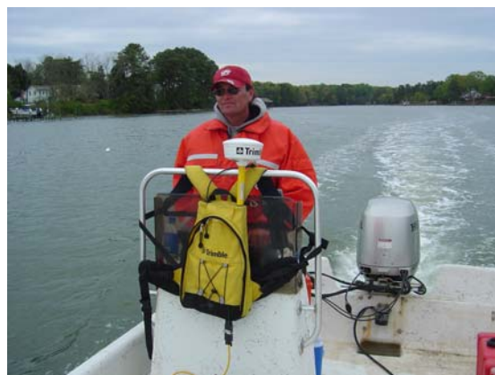
Figure 29. Mapping shoreline features from a boat with GPS equipment driven parallel to the shore.
