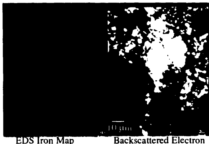
Figure 6.3: SEM and EDS images of iron polyimide composite.
