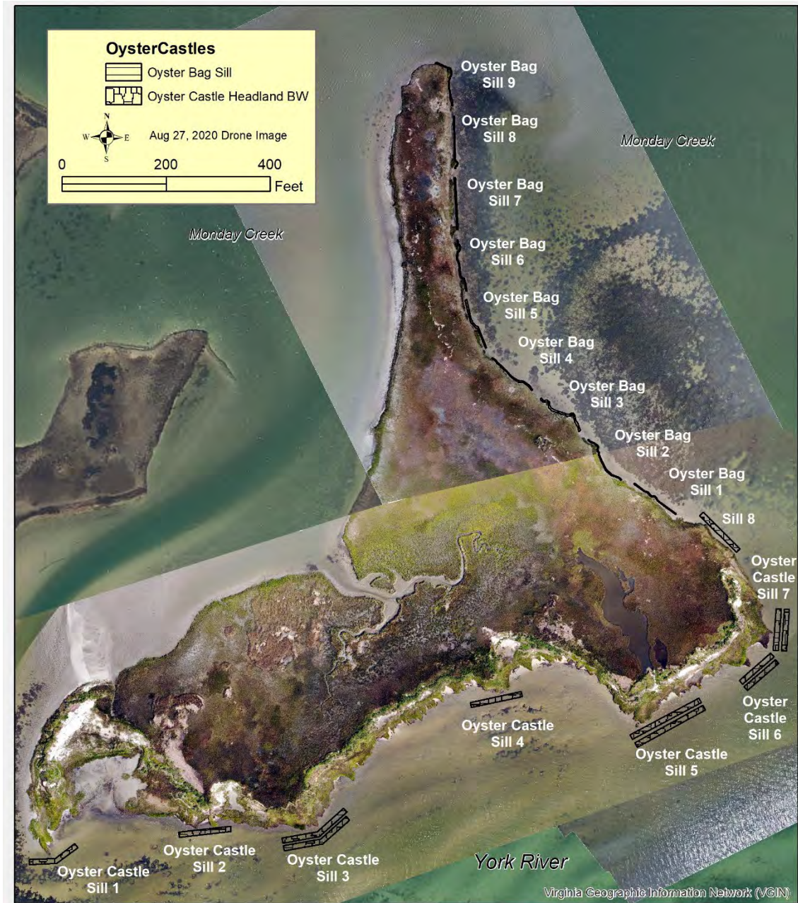
Figure 9. Proposed living shoreline project at Hog Island using oyster castles and oyster bags to create living sills along the shoreline for habitat restoration and shoreline protection.
