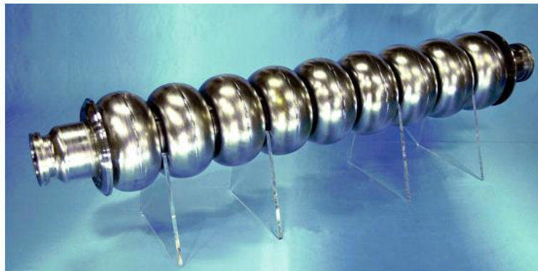
Figure 1.5: 9-Cell Nb SRF accelerator cavity, from JLab.org
