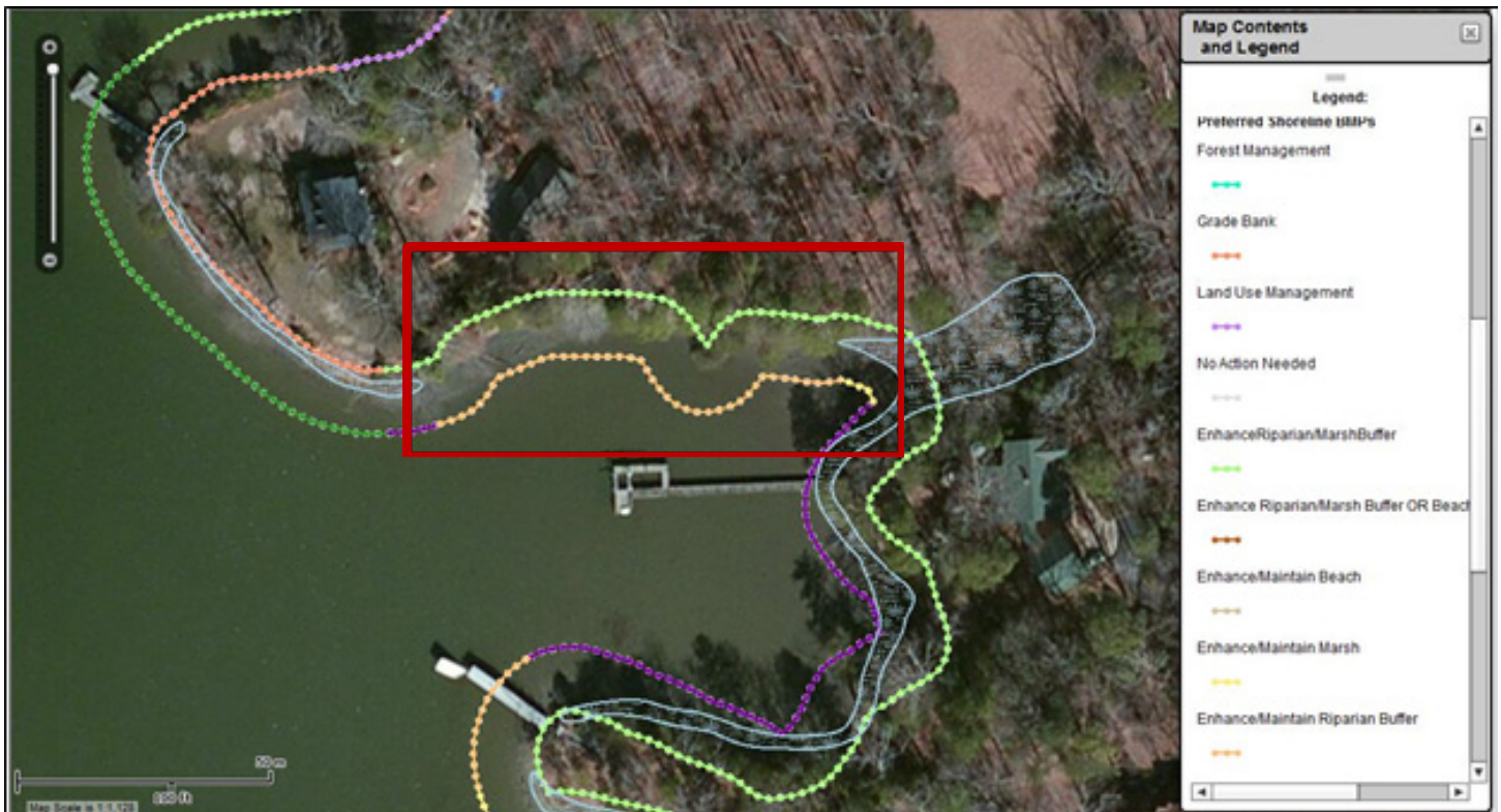
Figure 2. Recommended Shoreline Best Management Practices along Virginia Marsh's property as reported in the CCRMP
